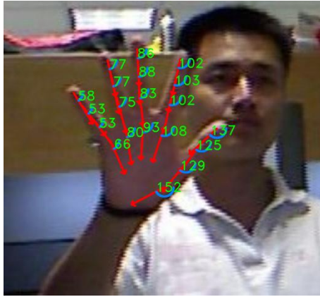
Fig. 5. Finger segments shown running from S_{i+1} to S_i and each segment’s angle from the horizontal.
