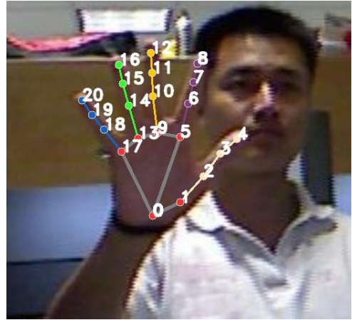
Fig. 3. A cropped image from the SVM training data [14] annotated with MediaPipe Hands keypoints and their indices.
